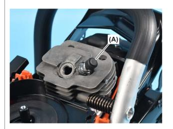
1. Before testing crankcase and cylinder leakage, remove decompression valve (A) from cylinder.
