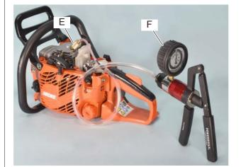
**NOTE:** Do not exceed 30 kPa (0.3 kgf/cm<sup>2</sup>) (4.3 psi). Otherwise, damage to the oil seal may occur.
