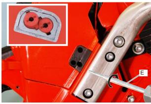
3. Remove the tool from limiter cap by turning clockwise, leaving the limiter cap in place.
